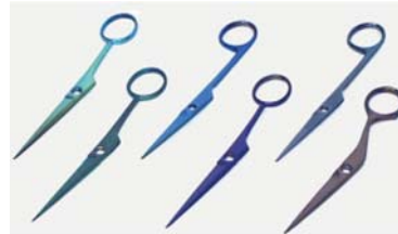
Figure 9: Examples for decorative coatings with different colours based on AlTiN.
